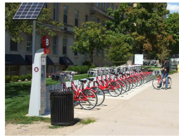
Typical bike share station with steel plates and electromagnetic docking points (Madison B-Cycle)
