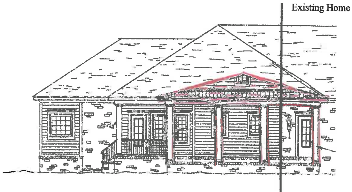
Proposed addition side view of 1410 Geiger Avenue with staff recommendations in red for hipped carport roof
