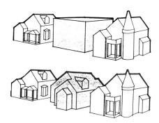
Do not construct buildings that disrupt the scale of the street. Break up box-like forms into smaller varied masses.
