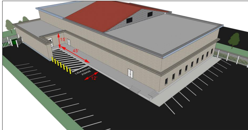
Figure 27-5.211.C: Loading Area Configuration
