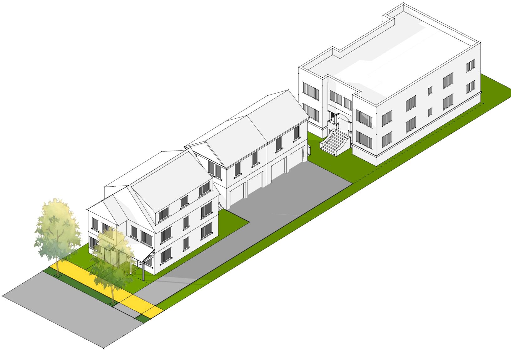
Above: Triplex + ADUs + Multiplex Small; Example of multiple Missing Middle Housing types on a deep lot.
